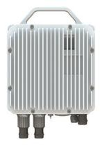
*DMR-X-ST* is a single-transceiver all outdoor, IP radio system operating from 6GHz to 42GHz, modulations to 4096QAM, and ultrawide bandwidth operation to 112MHz ETSI and 160MHz ANSI. *DMR-X-ST* can achieve capacities up to 2.75Gbps per radio without compression.
